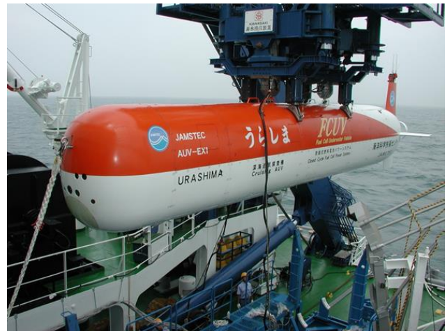
Fig. 1. Deep-sea cruising AUV Urashima
