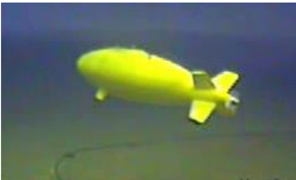
Fig. 6 Zig-zag cruising test
